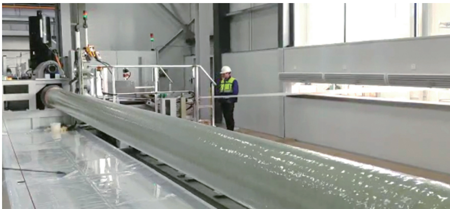
◎ 13 米德国进口四轴联动缠绕机 13-meter Germany imported four-axis linkage winding machine
