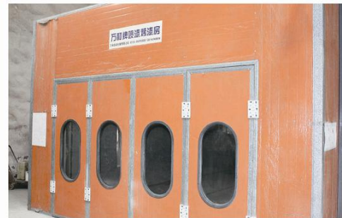
烤漆房 Curing Chamber
